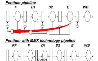
Figure 2. Pentium Processor and Pentium Processor With MMX Technology Pipeline
