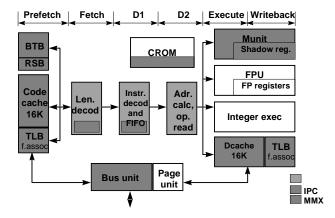
Figure 5. Block Diagram of the Pentium Processor With MMX Technology
