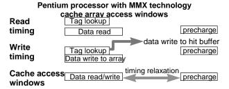
Figure 4. Pentium Processor With MMX Technology's Cache Array Access Windows Architecture
