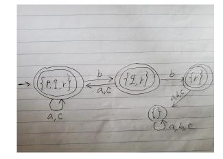
The state state is  $\{p,q,r\}$  and the final states are  $\{p,q,r\}$ ,  $\{q,r\}$  and  $\{r\}$ .
