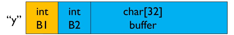
The code allows assignment of field B1 of y, which corresponds to field c of x
