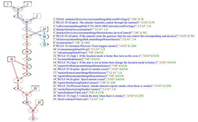
Fig. 3: IoT attack graph example. The meaning, type, and probability of each node are shown on the right.
