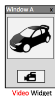
Figure 3: A photo capturing application presents a video camera widget, instead of a camera widget, to trick the user into also granting access to the microphone. The windowing display context surrounding the widget shows a camera preview for photo capturing.
