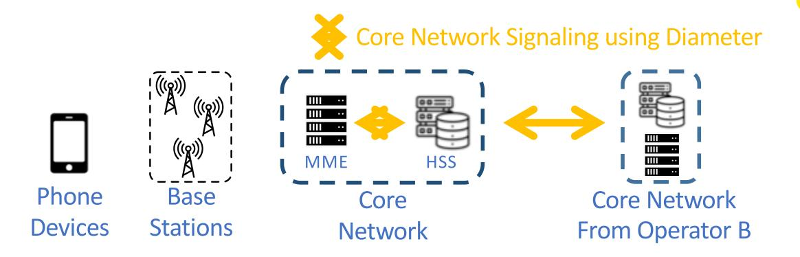
Signaling messages are exchanged between Core Network components for session management, mobility support, etc.
